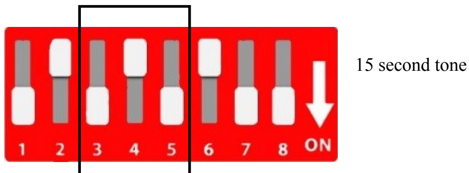
FIGURE 4 Dip switch sw3,4&5 configuration
