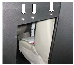
**Step 14 Mounting Sliding Doors on Slides** Carefully slide the door panels on the Slides. Ensure smooth movement and latch functioning.
