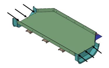
**Step 3 Rear Panel to Bottom Trays and the walls**
