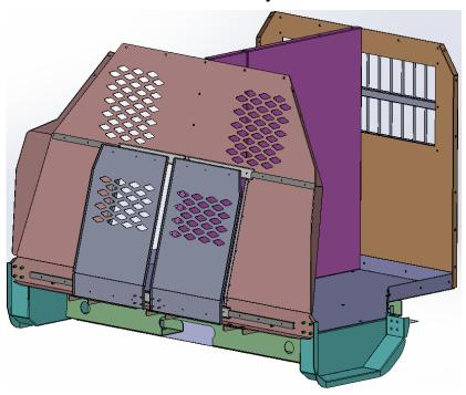
**Step 4 Top Cover Panel to Rear and Front Panel, and Side Panel's Covers**
