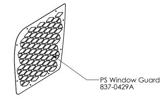
INSTALLATION HARDWARE: 28x - 837-0148A Window guard Mnt Brackets 28x - #10 Self Tapping Screw 28x - #10-32 5/8" Round Screw 28x - # !0-32 Nylock Nut 28x - #10 Flat Washers
