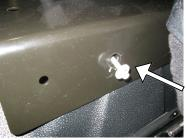
NOTE: Do not reuse the 2 rear factory plate mounting bolts.
