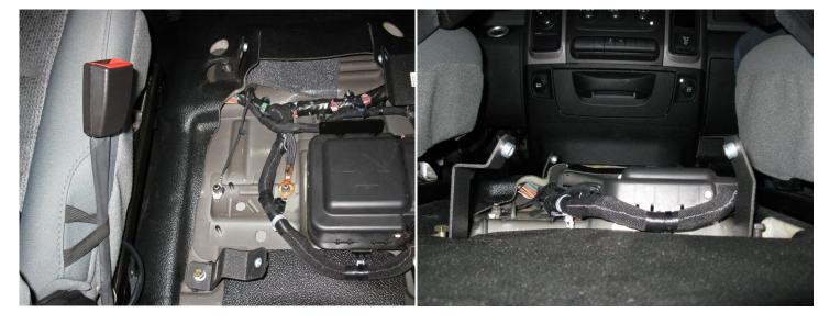
Step 5 Places Floor plate over mounting bracket and attach floor plate using supplied 3/8-16 Hex bolt . For easy assembly tighten these four bolts before tightening factory floor bolts.
