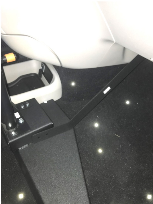
21) Place the OEM hex flange nut on to the left most bolt just enough for the threads to bite, giving 806-1508A strap2 lots of play to move.
