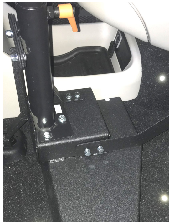
22) Use two (2) 1/4-20 x 3/4 Hex Bolt s with two (2) 1/4-20 lock washers to hand tight fasten 806-1508A strap2 to 806-1506A LT6600 Grand Caravan Base. A socket wrench may be needed to push the 806-1508A strap2 into place.
