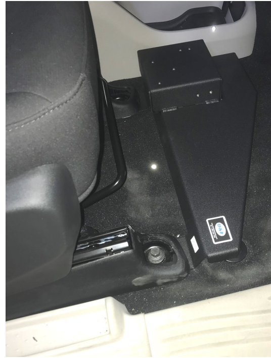
8) Install the front right 15 millimeter bolt hand-tight, leaving the ability to adjust the position of the 806-1506A LT6600 Grand Caravan base.
