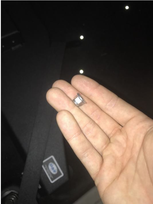
19) Use a ten (10) millimeter wrench to remove the OEM hex flange nut found under glove box.
