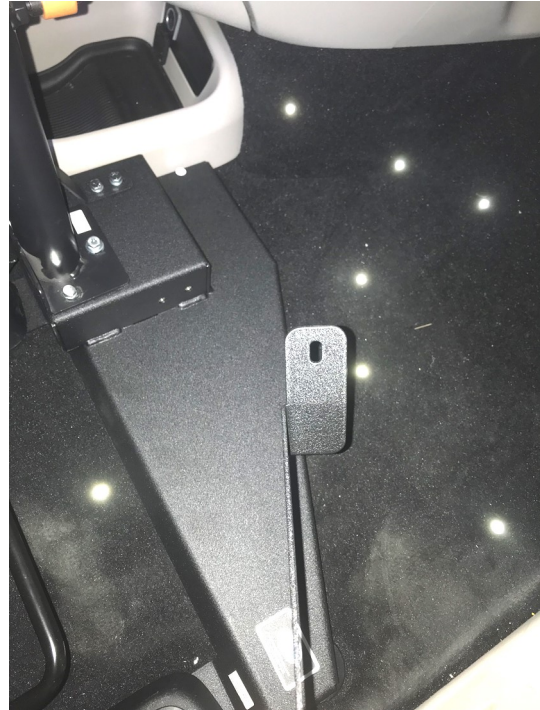
20) Place 806-1508A strap2 over the left most OEM bolt seen in step 18.
