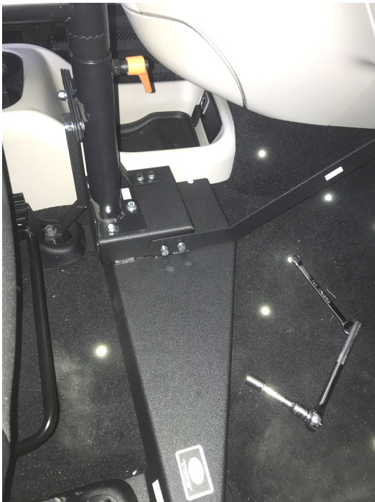
23) Install Front left fifteen (15) millimeter bolt fastening down 806-1507A strap1 & 806-1506A LT6600 Grand Caravan to the vehicle floor.
