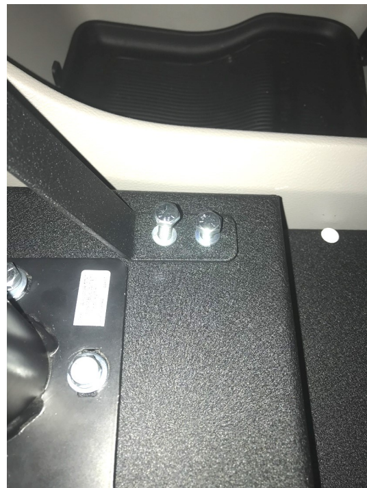
16) Use two (2) 1/4-20 x 3/4 Hex bolts to fasten (hand tight) 806-1479A LT Strap1 to 806-1506A LT6600 Grand Caravan Base.
