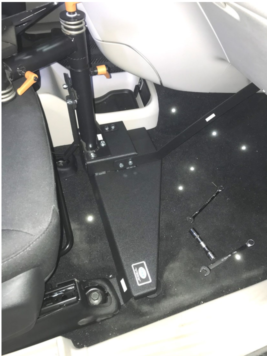
23) Install Front left fifteen (15) millimeter bolt fastening down 806-1507A strap1 & 806-1506A LT6600 Grand Caravan to the vehicle floor.
