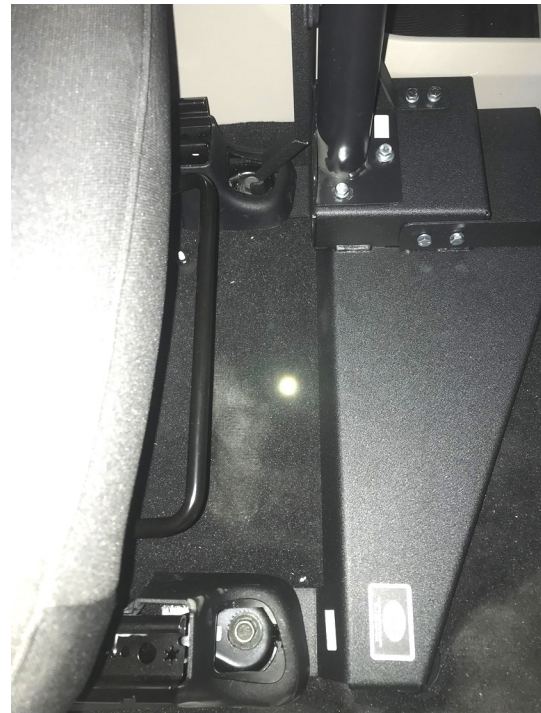
24) Fasten down all 17 bolts including the four Torx in the seat plastic foot covers and the two (2) fifteen (15) millimeter rear seat bolts.
