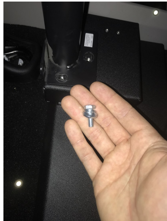
10) Install three (3) (hand-tight) 1/4 -20 3/4 Hex Bolts with three (3) 1/4 20 lock washers and three (3) 1/4-20 flat washer (one per bolt).
