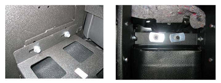
Step 9 Slide console forward tight to dash and tighten the 4 front bolt and the 2 rear bolts.
