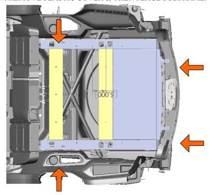
Insert Hardware to secure sub frame where marked above.
