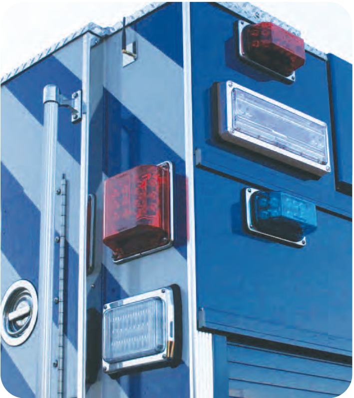
AC surface mount model SPA260 requires a 6 3/8" w x 4 11/16" h cut-out
