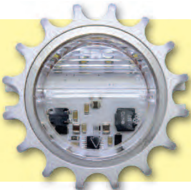
LED100 - Q01 Compartment Light with glare reducing lens
