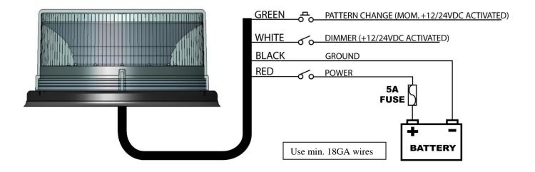
RED – Connect to POSITIVE terminal of a +12/24V BATTERY through a SPST switch and a 5A fuse BLACK – Connect to GROUND terminal of a +12/24V BATTERY. WHITE – Connect to +12/24VDC through an ON/OFF SPST switch. GREEN – Connect to +12/24VDC through a Normally Open MOMENTARY switch.
