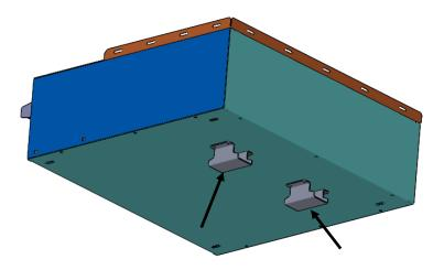
Step 7 Slide in the cabinet and locate the rear holding brackets against the channel on the subframe.
