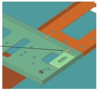
Note locations of reference notches to ensure proper assembly.
