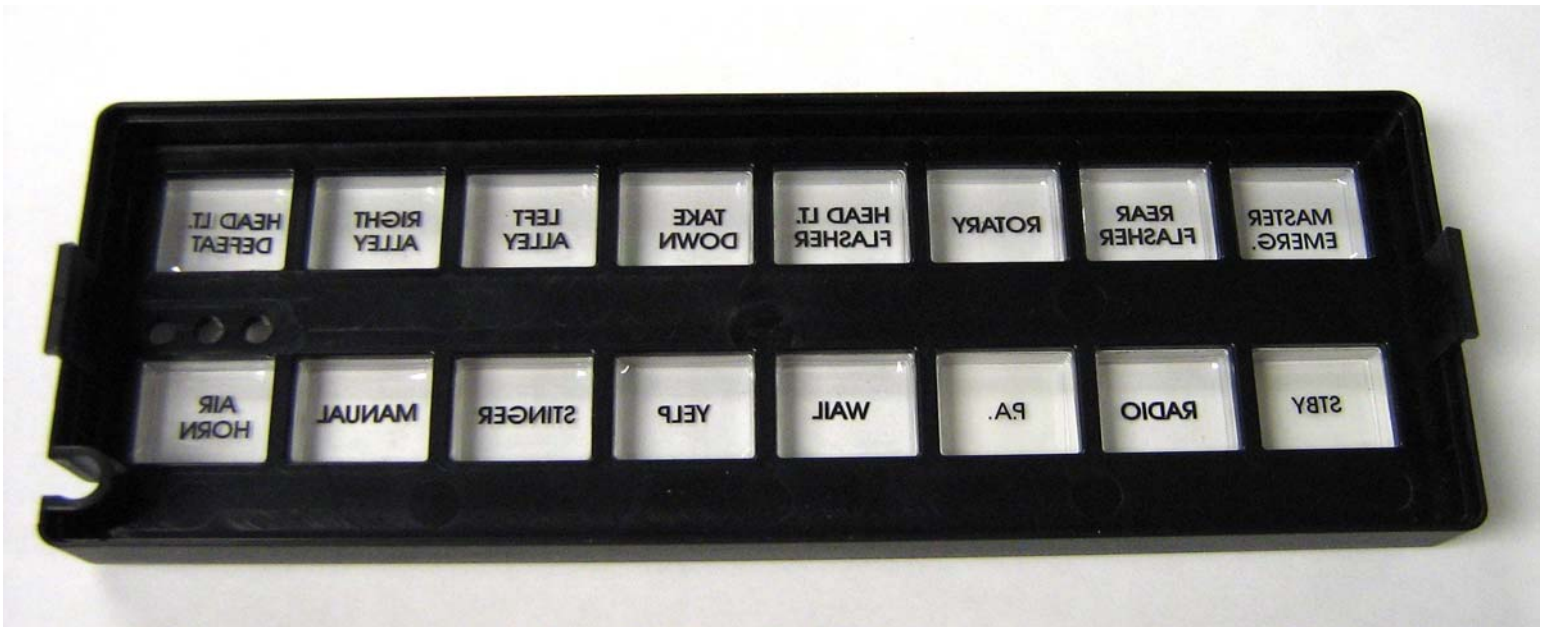
Figure 5b - Touch Panel Label Positioning
