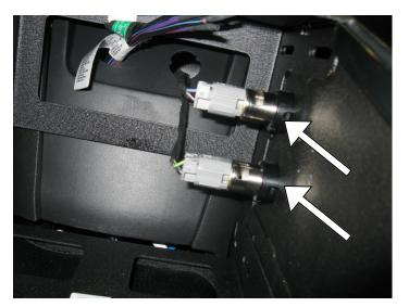
Attach console to both, front and back, mounting brackets using supplied hardware.
