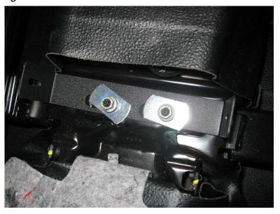
Step 6 Mount the front console bracket using bolts removed in Step 3. Using the console as reference, center the bracket and tighten the bolts.
