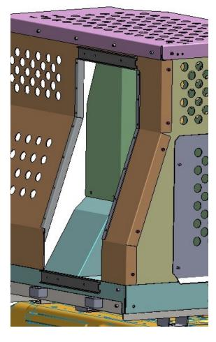
**Step 9 Inner Slides and Latch to Front Door**
