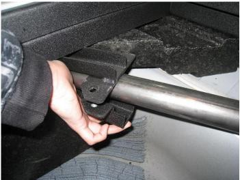
6. Install the *cabinet*. To secure the *cabinet* from sliding, install two ¾ *star knobs at the side of the* 934-0518 *cabinet*.
