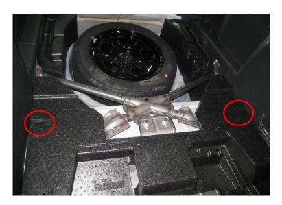
2. Install the *933-0113A liftable subframe* and secure using the *factory bolt* and *sleeve* removed in step 1. Install a *fender washer* on to the *sleeve*.
