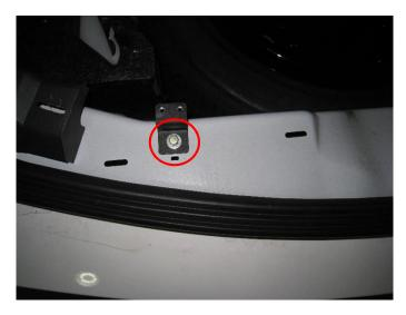
4. Use two #10 screws with a washer to secure the bracket on the sill to the bracket on the 9330113A liftable subframe.
