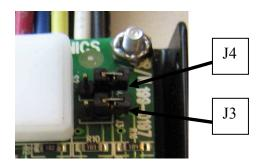
J3 and/or J4 OPEN (like in the picture) it will set Switch 1 and/or Switch 2 as ON/OFF switch
