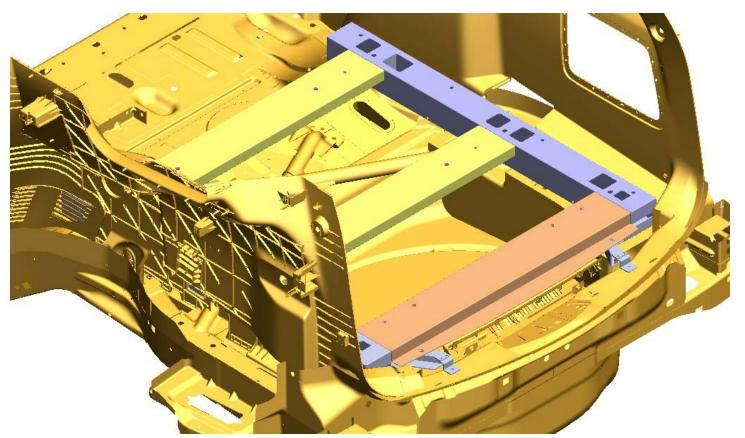
Step 4 Side Cover Panel Place Side Cover Panel Over the Sub-Frame and Secure using hardware provided.
