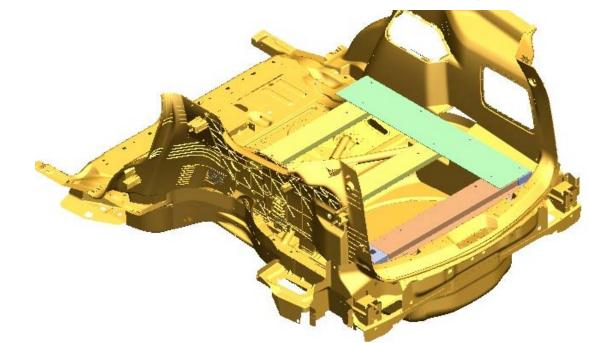
Step 5 Cabinet on Sub-frame Place Cabinet on Sub-frame and secure using hardware provided.
