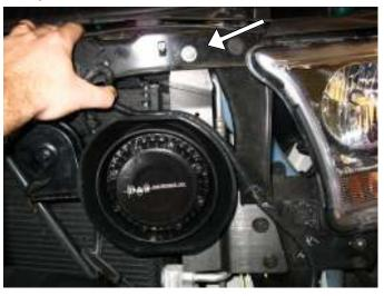
Install speaker bracket with to front rad support. Attached top of bracket behind rad sup-
