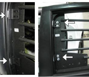
Step 3 Adjust the window bar and then tighten hardware from step 2.
