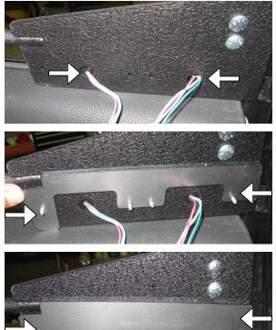
Step 6 (For Optional Light Kit) Secure lights and plates using hardware, line 4 & 5.
