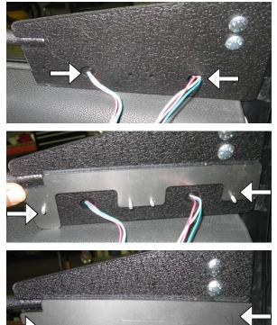
Step 6 (For Optional Light Kit) Secure lights and plates using hardware, line 4 & 5.
