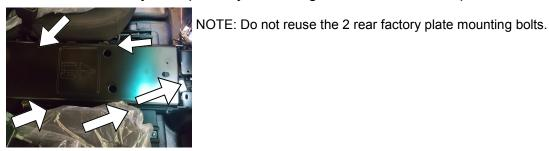
Step 2 Unclip wiring from floor plate, before removing plate from car.
