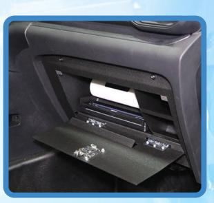
This unique design allows you to mount your printer in the glove box space by simply removing the factory glove box and installing the D&R model printer holder, with no modifications required, and mounts directly to the vehicle by using existing OEM mounting points.
