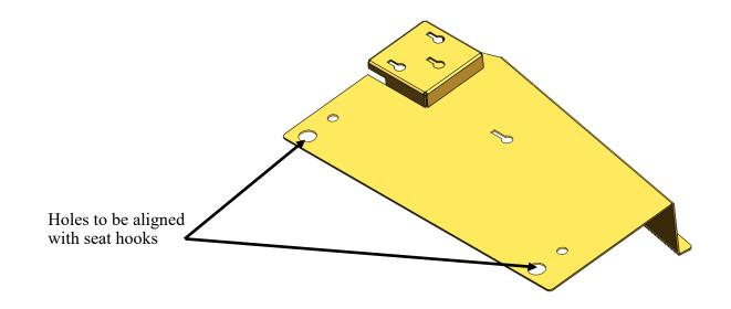
Follow the drawing on the next page for securing the brackets to the floor mount.
