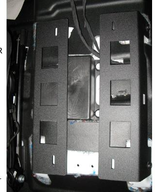
Step 8 Center the console to the floor mount brackets and secure using 4x hardware line 1,2 and 3. Step 9 (For Optional Side Pocket) Place the DS or PS Console Side Pocket on the console and secure using 6x (Each) hardware line 5,6 & 7.
