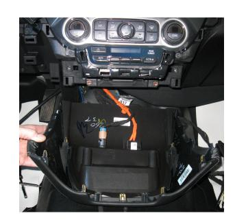
Step 2 Unplug and Remove the 12V and 110V Power outlets. Caution! Do not use excessive force.
