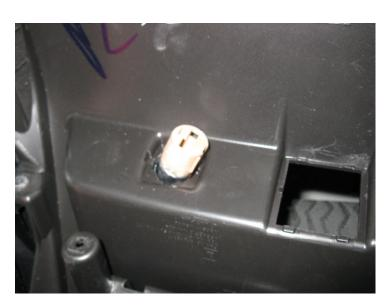
Step 3 Insert both the Power outlets on the D&R Console. Note separate the plastic casing on the 12V outlet for easy install.
