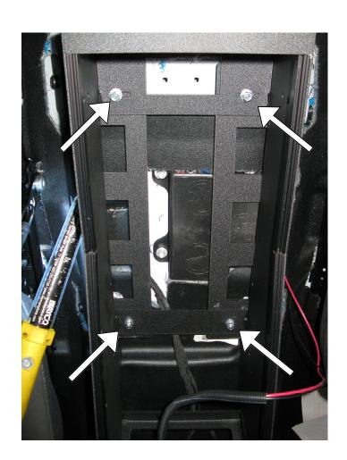
Place the DS or PS Console Side Pocket on the console and secure using 6x (Each) hardware line 5,6 & 7.
