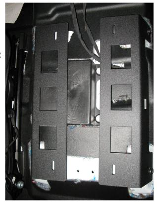
Step 6 Place the Console in position and reconnect the 12V and 110V Power outlets.
