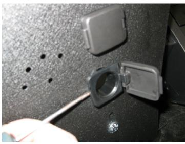
**CAUTION**: DO NOT hammer or force the plastic covers. They have a pin on each side, that must be pressed using a small flat-head screwdriver when installing.
