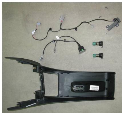
Step 5 Install antenna on console using screws obtained from Step 4. Install sockets and outlets as shown.
