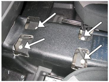
Step 4 Attach rear brace mounting brackets provided. Using (x2) hardware line 2 & 4. (Do not tighten) the bracket to body of the car.
