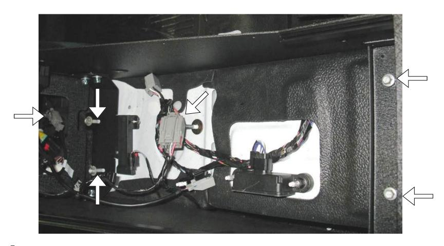
Step 7 Install DS & PS wings using 2 sets each of hardware, line no. 1 & 2. Adjust the height of console and tighten all nuts to secure.
