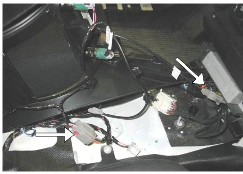
Step 4 Remove Key Antenna, 12V outlets and USB/Aux outlet. Remove the harness completely. Retain screws for Step 5.
