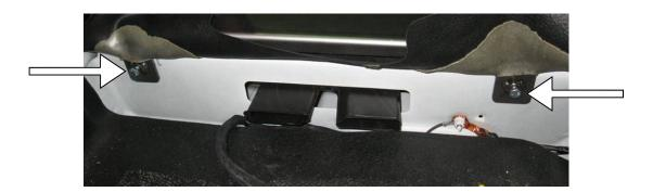
Step 5 Install mounting strap provided using 1 set of hardware, line 2, 3 & 4.
