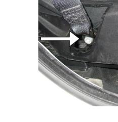
Step 4 Install floor mount in vehicle using hardware, line no. 1
