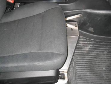
Step 7 (For Optional LT6600) Place LT6600 over the floor mount and secure with mount and strap using 4 sets of hardware, lines 2,3 & 4.
