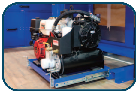
CUSTOM SLIDE-OUT TRAY FOR AIR COMPRESSOR
